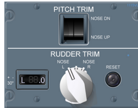
PITCH TRIM & RUDDER TRIM Panel
