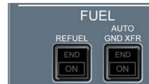
Refuel/Ground Transfer Panel
